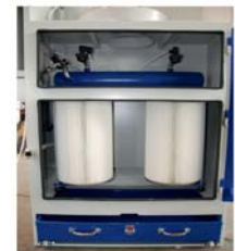
Integrated suction with cartridge filter 0,75 kW with dust drawer
